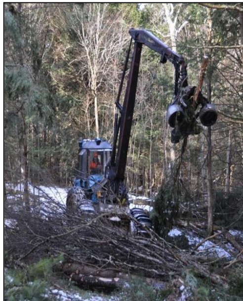
Manual and cut-to-length harvesting affords opportunities to enhance forest floor structure by topping and delimiting at the stump. Harvests conducted by feller-buncher call for other approaches to retain debris on site, including retaining low-quality standing trees. Photo by Bill Stack.
